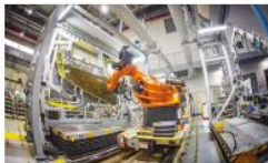
Wing Assembly Automation with Robotic Drilling Systems(RDS)
