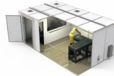
FULLY ANECHOIC CHAMBER
