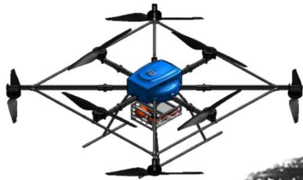
Fire Hydrant Drone (powder type)
