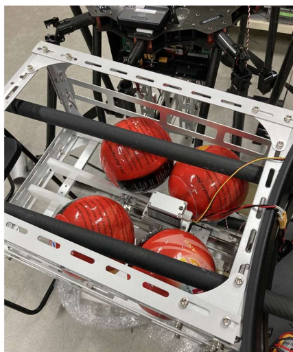
Fire Extinguishing Ball Mounted
